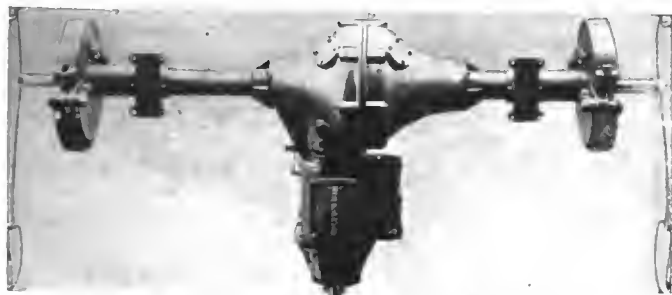
Rear Axle and Transmission Unit Is Distinctive
